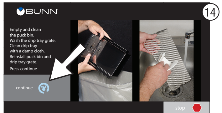
Empty and clean the puck bin. Wash the drip tray grate. Clean drip tray with a damp cloth. Reinstall puck bin and drip tray grate. Then press “continue” button.
