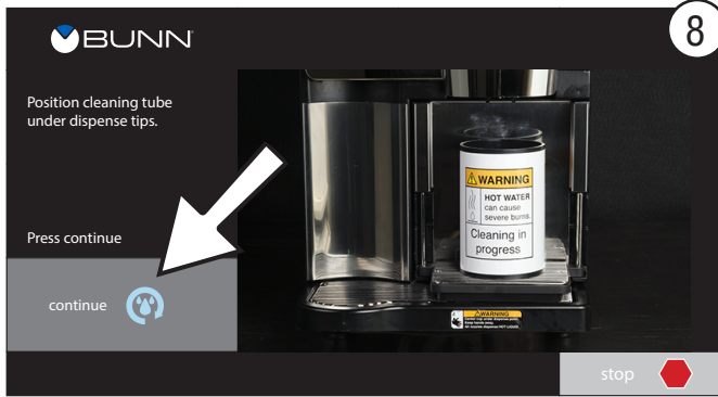
Position cleaning tube under dispense tips. Then press the “continue” button.
