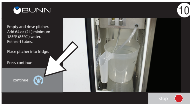
Empty and rinse pitcher. Add 64 oz. (2L) minimum 185° F (85° C) water. Reinsert tubes. Place pitcher into the fridge. Then press the “continue” button.
