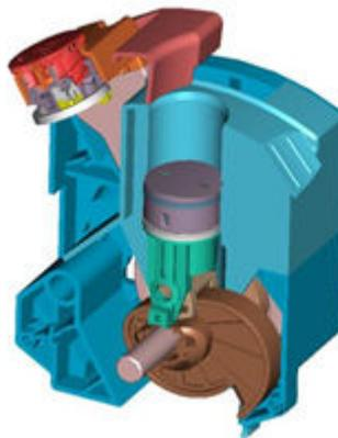
**Waste wipe** The brewer runs through, herewith the lower piston moves to the top position. Now the brewer starts running clockwise and the coffee cake is swiped from the piston into the waste bucket.
