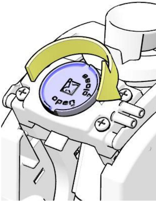
1. To remove the filter head, turn the knob clockwise.
