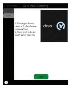
Using a clean cloth, wipe the touch panel free of any contaminants. The screen will be deactivated for 15 seconds to complete this action
