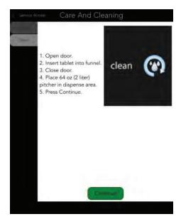
The machine will now complete the cleaning cycle by passing hot water over the tablets in the funnel, dissolving them. This creates a cleaning solution designed to break up the oil residue created in the coffee making process. A status bar will indicate the cleaning cycle progress on the screen.
