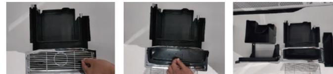
Wash the grid, waste water anti-sprinkling board, drip plate under the faucet thoroughly with a brush and wipe it with a towel, reload the dry drip tray assembly into the machine and confirm that it is in place.
