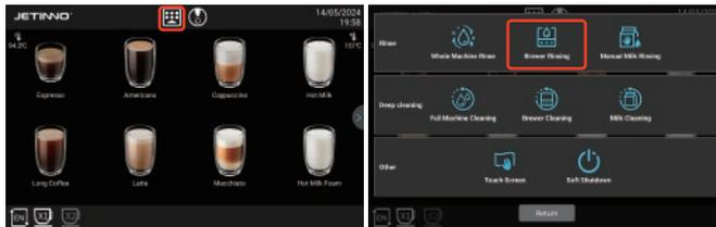
In the pop-up box, there are "OK" and "cancel" keys, click "OK" to execute the washing procedure, click "cancel" to return to the previous layer; click "OK" button, the machine is cleaning, please wait..., after completion, the interface shows: finished cleaning, click "OK", return to the order interface.
