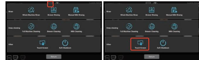
Click the "Quick Maintenance Menu" button, and in the pop-up interface, click the "Touch Screen" option. After locking the screen, wipe the screen with a soft cloth.
