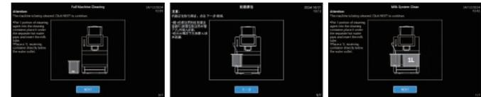
Follow the screen, place 1 piece of cleaning agent into the cleaning container, place it under the independent hot water pipe and insert the milk tube; place the 1L water container under the outlet nozzle and click "Next";
