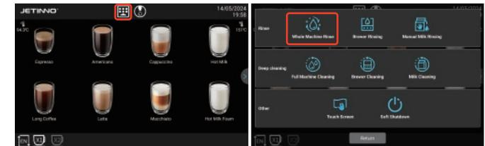
Click the "Quick Maintenance menu button" button, and click the "complete machine flush" option in the pop-up interface.
