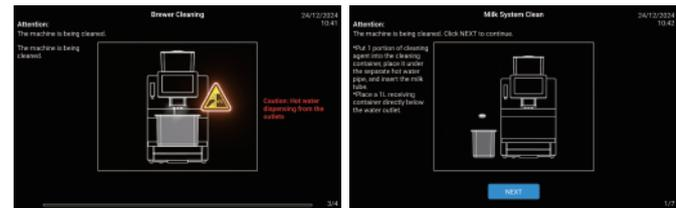
The machine is performing the cleaning process. In the process of cleaning, please wait later. After the progress bar is complete, proceed to the next interface. After the system is cleaned, remove the cleaning box, insert the milk tube into the refrigerator interface, put it in the milk box, close the refrigerator door, click the "OK" button on the interface, and return to the upper menu.
