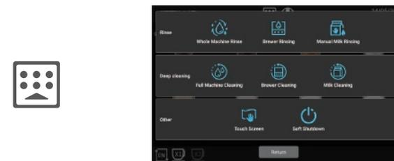
Quick maintenance menu key includes: washing (machine washing, brewer washing, manual milk washing), deep cleaning (machine cleaning, brewer cleaning, milk road cleaning), other (touch screen, soft shutdown), functions.
